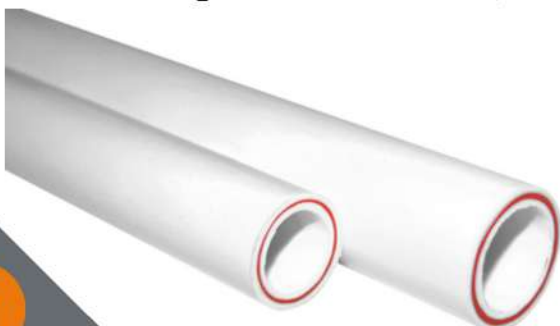
PP-R Glass Fiber Reinforced Pipe - PN20 - SDR7,4
